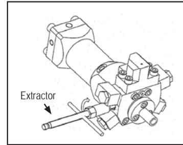
4. **Disassemble the orifice nozzle for cleaning.**
