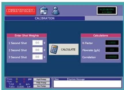
When the Pour button is pushed during calibration, only the selected component will be dispensed. The other component will continue to circulate at low pressure from the pump, through the diverter valve and heat exchanger, back to the tank.
