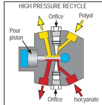
4. **Adjust the orifices in or out until you see the desired pressure on each chemical high-pressure gauge.**
