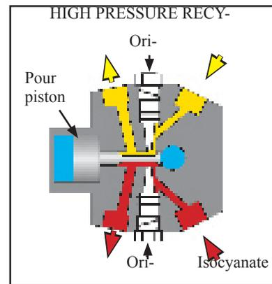
**6. Adjust the mixhead orifices to the required pressure.**
