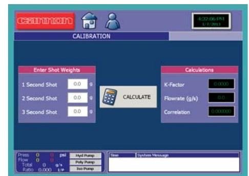
To check individual pump throughput, select either the ISO or Poly calibrate. Follow the procedure for calibrate, using 1, 2, and 3 second shots, weighing each shot.
